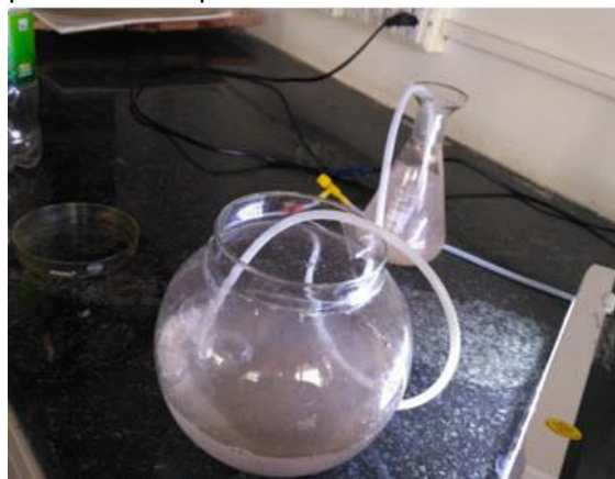
Figure 4.1: Brine shrimp lethality assay (BSLA) set-up
